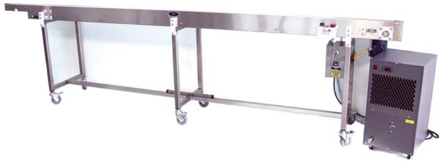
6' Cooling Conveyor For Pre Bottomed Chocolates
